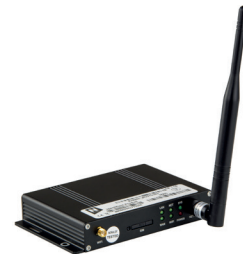
IGSM4G/IP router modem Only required if 4G aerial needs to go on roof, max 80 metres from IPGUARD (usually in top floor riser), ZAN1055 and AR122 PSU included.
