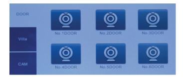
Panels & IP Cameras – monitoring all Panels and IP Cameras setup to the system from IPVIEW Monitor Interface. Can trigger Unlock function and take real time snapshot saved into the internal or external (MicroSD card)
